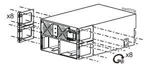
2 Install the rails. Follow the rail installation instruction in the rail kit.
