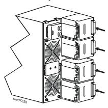
2 After the UPS is hardwired to branch circuit mains, complete steps 2-5.Connect all four battery modules.
