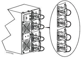
**3** Reinstall the battery compartment doors. Tighten the thumbscrews to secure the doors.
